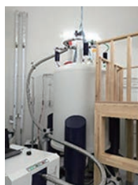
800 MHz superconducting nuclear magnetic resonance equipment
