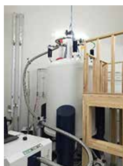
800 MHz superconducting nuclear magnetic resonance equipment
