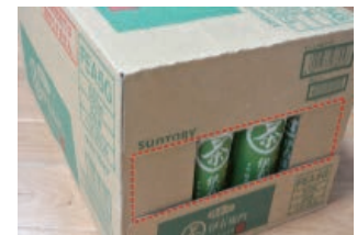
Short flap cardboard cartons that reduce cardboard usage on its sides
