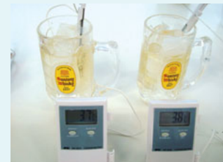
Liquid temperature-change test for a highball mug
