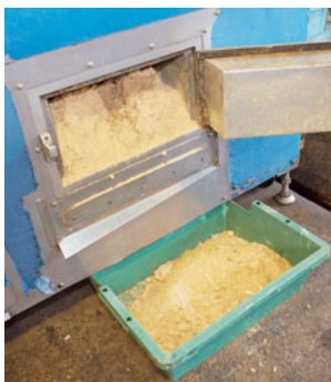
Coffee grounds collected by designated waste management providers are compressed and fermented while being mixed in a large, high-speed fermentation compost machine, which turns the grounds into a fine, powdery raw material for compost.
