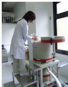
An inspection utilizing a germanium detector
