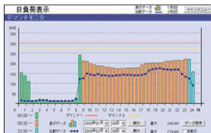
Monitoring power usage during different time zones with a demand monitor
